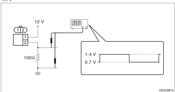
5) Replace the ABS wheel speed sensor if the inspection result is not within the standard value.
